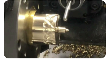
Live-tool milling on a turned part
