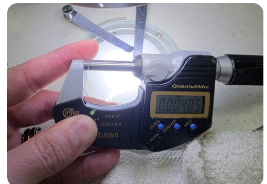
Mitutoyo QuantuMike digital micrometer at the bench
